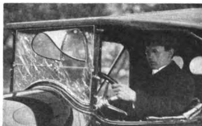
Frey U-Can-C rain shield as it appears mounted on the glass windshield
